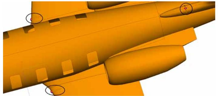
Placement of the three notch antennas
