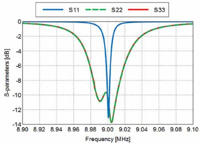
The bandwidth after matching is sufficient for practical usage
