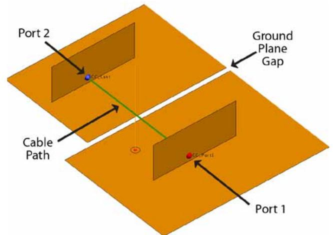
Shielded RG58 cable above ground plane with gap
