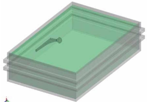
Hip implant in ASTM phantom
