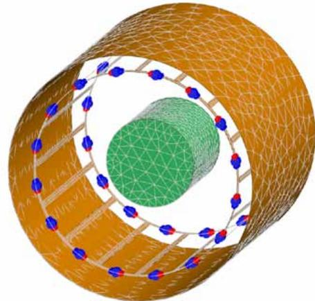
"Birdcage" coil with cylindrical phantom and shield
