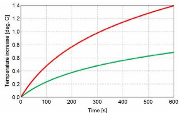
Hot-spot temperature as a function of time at two different power levels: 40 W (red) and 20 W (green)
