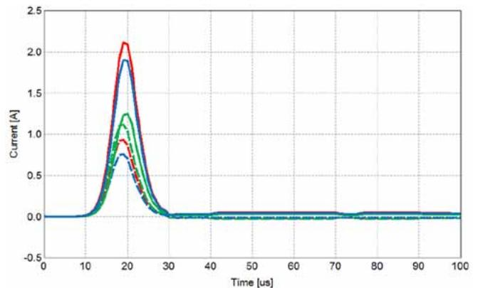
The currents at three cable terminals caused by lightning stroke; metal fuselage (dotted lines) and CFRC fuselage (solid lines)
