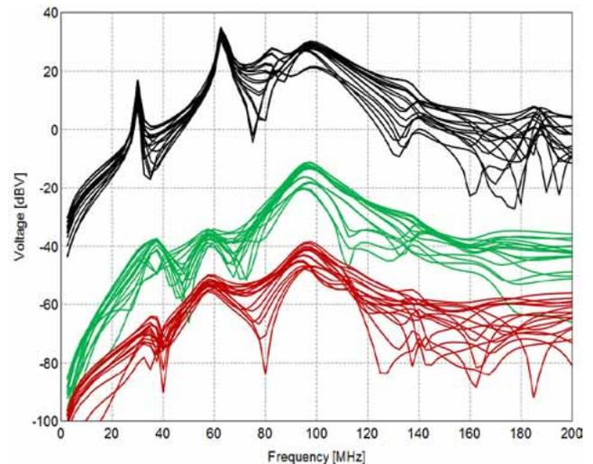
Typical voltages at the cable terminals for different fuselage materials. Black: plexiglass; green: CFRC material; red: metal.
