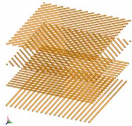
Carbon fiber arrangement in the composite material
