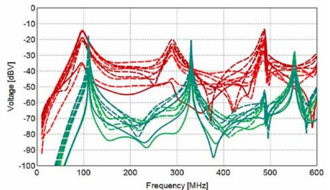
HIRF-induced voltages at the terminals of the cables. Red: unshielded cable harness; green: shielded cable harness
