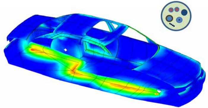
Surface currents caused by a radiating cable running along the inside of a car's bodywork. An example of a cable that can be modelled in FEKO (insert)
