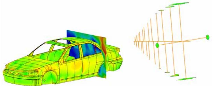
*The visualisation of near fields for a full vehicle illuminated by a log periodic antenna*
