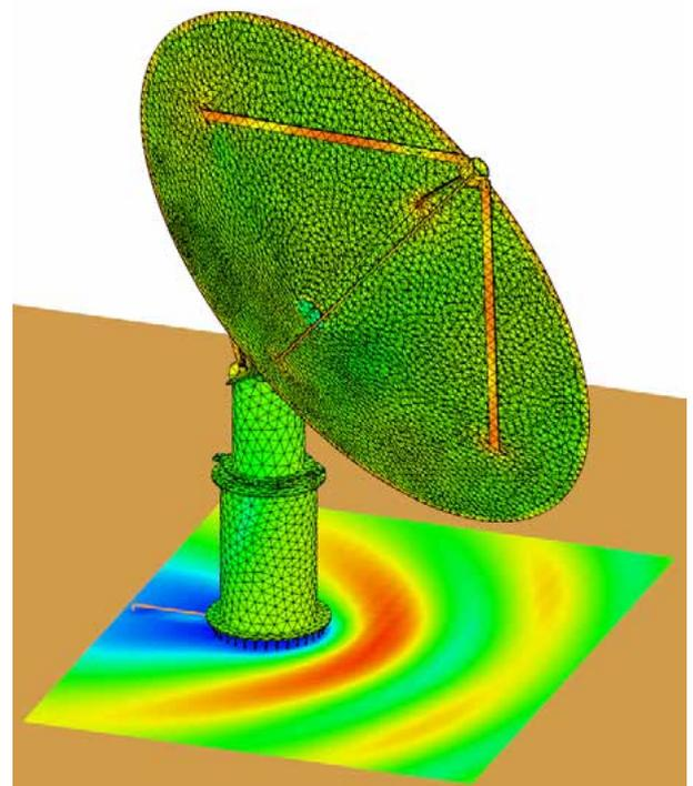
The surface currents and near fields during an indirect lightning strike on a scale model of the KAT-7 radio telescope (model courtesy of P.G. Wiid)
