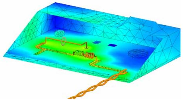
*The currents induced on a printed circuit board within an enclosure. The voltage to the PCB is supplied via a twisted pair of cables*
