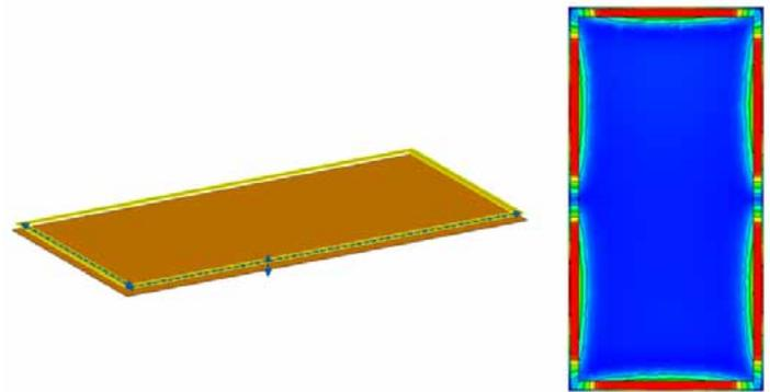
Display frame geometry tweaked using CMA to design a passive resonator
