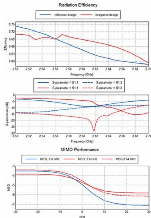
CMA optimised performance of antenna, display frame and battery compared to the reference design
