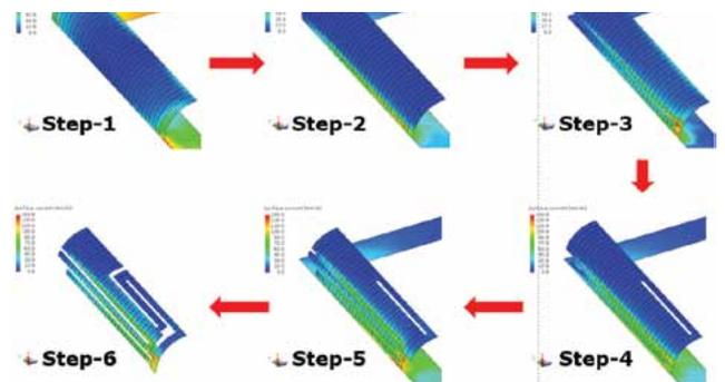
An antenna designed by systematically modifying a metal sheet based on the sheet's modal current distribution
