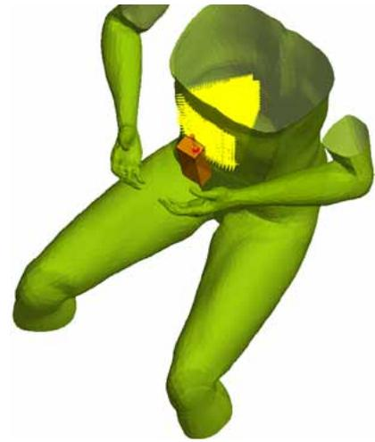
Phantom with radio close to body
