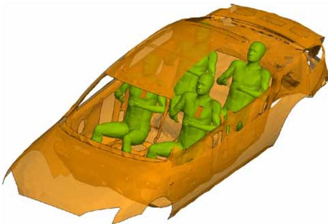
SAR computation for phantoms wearing personal radios in a vehicle
