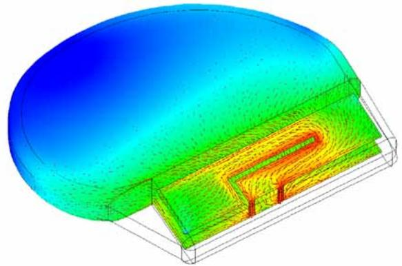
Surface current on a high gain planar inverted F antenna (PIFA) design (ISM band, 40 x 40 x 8 mm) for a cardiac pacemaker
