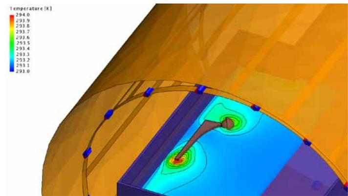
SAR distribution for the titanium hip implant placed in an ASTM phantom within a 1.5 T body coil (top). The resulting temperature distribution (bottom) after 10 minutes shows an increase of about 0.8 K at the tip of the implant
