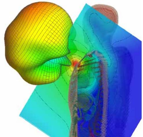
Pacemaker performance with anatomical model. The link budget indicates telemetry will be possible up to 10 m with a -31 dB source power
