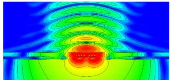
2.45 GHz simulation of injectable biosensor in a layered skin, fat, muscle phantom
