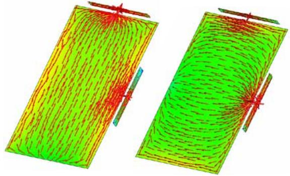
The placement of two MIMO elements is optimised with CMA to improve isolation [2]
