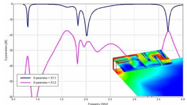
S-parameters of a novel quad-band MIMO antenna [1] for long term evolution (LTE) and WiFi
