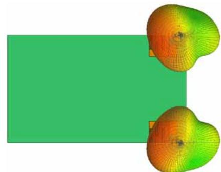
Far field radiation patterns for a novel quad-band MIMO antenna [1] for long term (LTE) and WiFi
