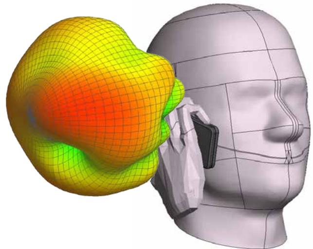
Far field radiation pattern at 1800 MHz. The model includes the mobile device, head and hand
