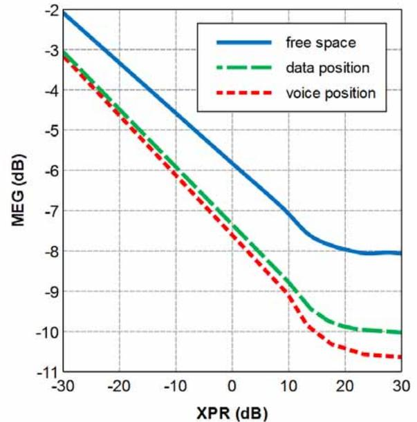
MEG at 3.65 GHz showing the drop in gain in the voice (against the head) and data (held with 2 hands) positions [1]
