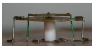
Christopher Thajudeen's design of a Dual Stacked Peano Top-Loaded Monopole. The figures show his schematic, the radiation pattern calculated using FEKO and photos of the antenna prototype (side and top view).
