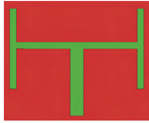
MoM with infinite planar dielectrics – Microstrip or stripline feed network.
