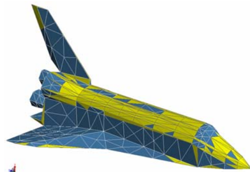
Figure 2: Distorted elements if geometry is meshed
