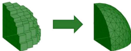
Cuboidal mesh elements (used before) and tetrahedral mesh elements (available in Suite 6.1) for the VEP solution of dielectrics.
