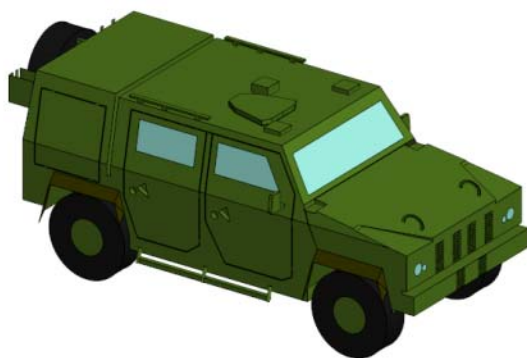
Miguel Sossouhounto’s CADFEKO model of a Light Multirole Vehicle (LMV).
